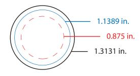
Imprint area INSIDE red dotted line. Blue line is for text or graphics that extend (bleed) all the way past the edge of the button. NOTHING IS TO BE OUTSIDE THIS LINE! Reference lines (blue and red lines) **DO NOT** print on your design. The black outside line and tick mark **WILL** be printed.
